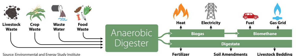
Figure 1: Anaerobic Digestion Process
